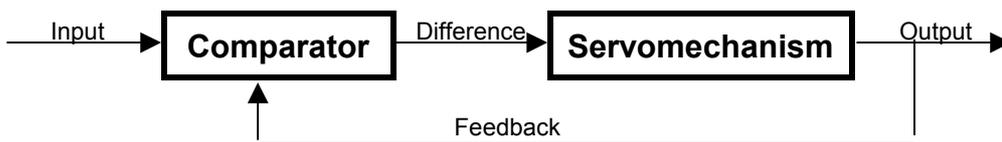
Figure 1 - The Basic Servomechanism
